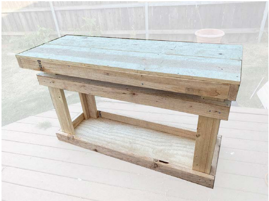
WORKBENCH. Built for needed flexible workspace during pandemic. Caster wheels and varnish were added. Height is appropriate to reduce lumbar strain while model-making and drawing. Narrow shelf is ideal for 18x24 paper storage. Lower shelf stores drill press and material organizers.
